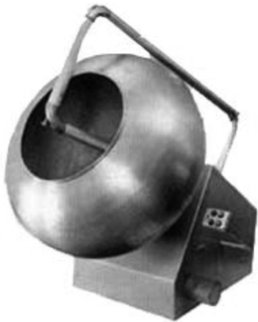
Fig. 32.8 • Traditional sugar-coating pan.
