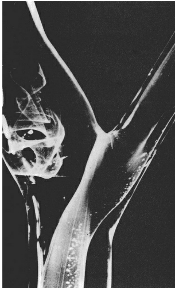
Figure 26-4 Glass model of the carotid bifurcation. Hydrogen gas bubbles show the streamlining of flow fields at the carotid flow divider and the complex counterrotating helical pattern at the arterial wall opposite the flow divider. (Reprinted from Zarins CK, Glagov S. Arterial wall pathology in atherosclerosis. In: Rutherford RB, ed. Vascular Surgery . 4th ed. Vol 1. Philadelphia, PA: WB Saunders; 1996:214. Copyright © 1996 Elsevier. With permission.)
