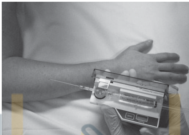
Figure 13–1. A slit catheter device used to measure compartment syndrome. (Reproduced, with permission, from Tintinalli J, et al. Tintinalli's Emergency Medicine: A Comprehensive Study Guide . 7th ed. New York, NY: McGraw-Hill; 2010:Fig. 275-6.)
