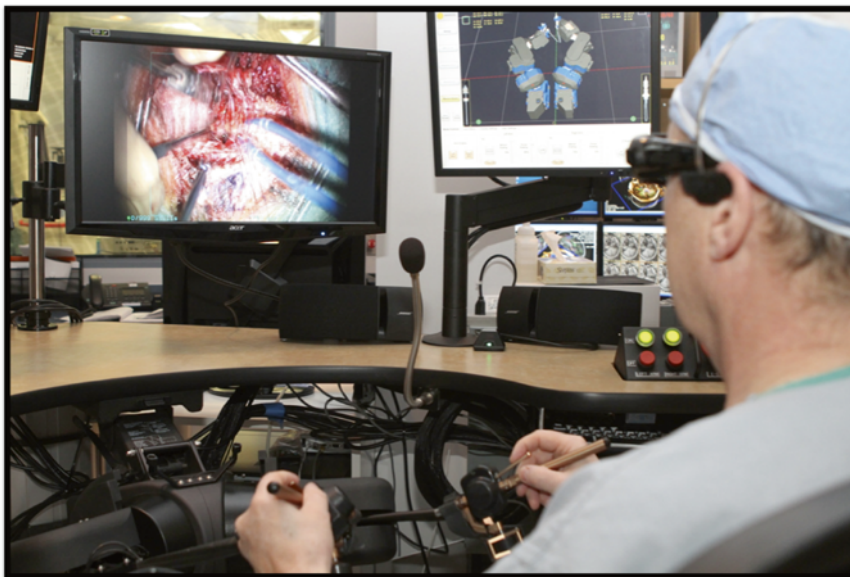
Fig. 4 The neuroArm human–machine interface recreates the sight, sound, and touch of the surgical site for the surgeon. The surgeon is provided with a 3D stereoscopic view of the surgical corridor. The command status display ( right of the stereoscopic display) shows the position of the neuroArm manipulators in relation to the radio frequency coil. The surgeon controls neuroArm using two modified PHANTOM hand controllers, providing 7 DOF control with 3 DOF force feedback. The surgeon communicates with the surgical team using a wireless headset
