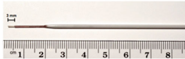
Fig. 1 Step-design cannula. The length of each infusion cannula was measured to ensure that the distal tip extended 3 mm beyond the length of the respective guide. This created a stepped design at the tip of the cannula to maximize fluid distribution during RCD procedures and minimize reflux along the cannula tract. We refer to this transition from fused silica tip to a fused silica sheath as the “step”
