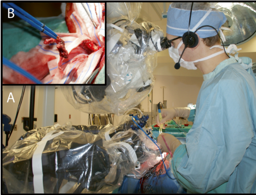
Fig. 5 (a) For microsurgical procedures, neuroArm is positioned at the operating table in the position of the primary surgeon. The assistant surgeon is able to operate in an ergonomic position relative to neuroArm and the operating microscope. (b) The neuroArm bipolar forceps can be used to coagulate, as well as remove pathological tissue
