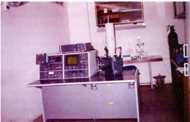
Figure 17.19: Scanning electron microscope used to study surface characteristics of the cells at very high magnifications upto 100,000 times
