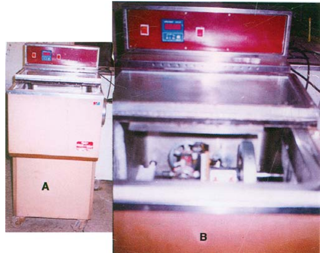
Figures 17.16A and B: Cryostat Microtomes: A. Outside view of cryostat used for cutting the frozen sections. B. Inside view of Freezing chamber of cryostat maintained at temperature of -25^{\circ}\text{C} in which microtome is fitted for cutting frozen sections
