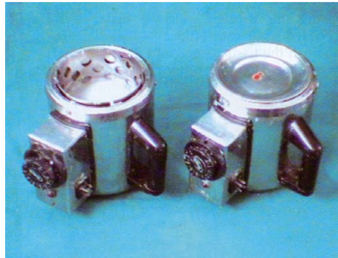
Figure 17.5: Automatic wax baths used for infiltration of wax into the tissues. The temperature of the wax baths is set at 65°C so that wax remains melted
