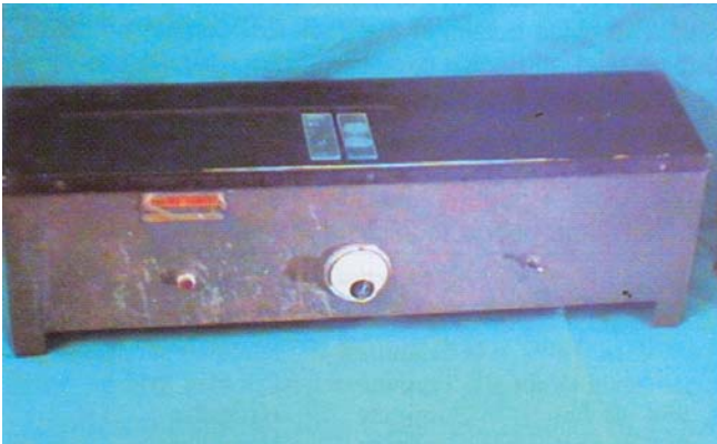
Figure 17.12: Slide warming table is used to dry the sections so that they get fixed to the slides
