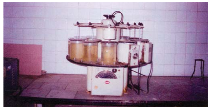
Figure 17.3: Automatic Tissue Processor: The different chemicals are filled in the glass jars. Two jars are filled with wax and the temperature of wax jars is fixed at 65°C. The tissue samples are automatically transferred from one chemical to another after desired prefixed time set on the dial
