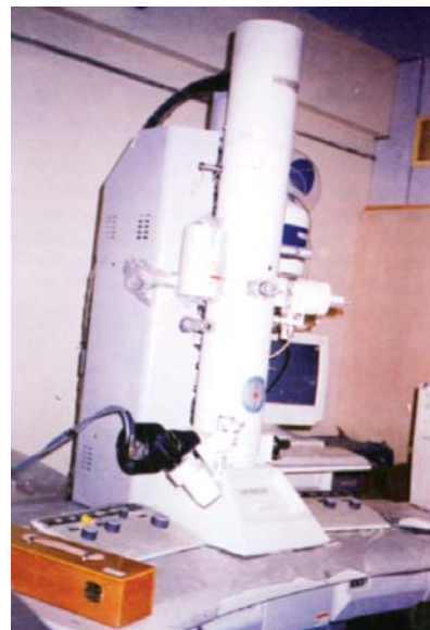
Figure 17.2: Transmission electron microscope used to study the subcellular structures at very high magnifications upto one lac times
