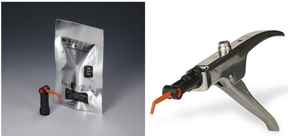
FIGURE 9-14 Single-unit auto-mix dispensing capsule for a two-paste resin-modified glass ionomer. The dispensing tip contains a mini static mixer for auto-mixing when expressed by a delivery gun device. (Courtesy of 3M ESPE Dental Products, St. Paul, MN).
