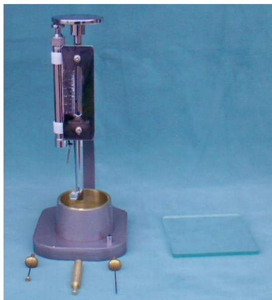
FIGURE 5.13 Vicat penetrometer used to determine initial setting time of gypsum products.
