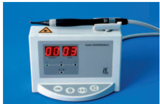
Figure 6.4 DIAGNOdent showing real-time and maximum (peak) digital display. The device consists of a probe, a fiber-optic lead, and a unit containing the electronics and the laser diode.
